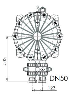
Inlet / outlet: DN50 nut 2"3/4
